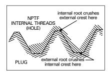
**PTF** fully formed Dryseal threads designed to achieve seal in tapped holes without need for sealing compounds.
